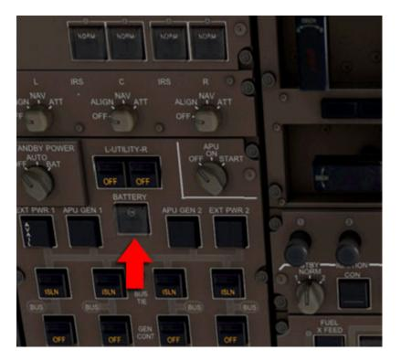
Left click to press the button to turn on the battery. The battery button has a protective cover over it that closes when the battery is turned on. If it is closed, you can right click to open it, then left click on the button to turn the battery off. Let's leave the cover closed so we don't accidentally turn it off. The battery should remain on at all times as it provides a backup power source to critical flight instruments.
