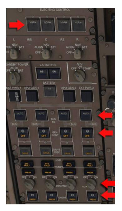
The ELEC ENG CONTROL switches allow the electrical system to operate the engines. These buttons also have guard covers, so right click if you need to open them and be sure to close the guard when you're done. The 747's engines are primarily controlled by electronic systems rather than hydraulic or pneumatic systems. If the electrical engine control system for an engine fails, you can click the button again to switch to an ALTN (alternate) electrical system.
