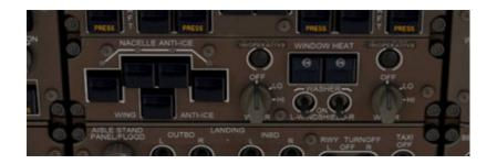
Nacelle anti-ice distributes air from the engines back onto the engine casing to slow formation of ice. Wing anti-ice distributes engine bleed air to the front of the wings. Both should only be enabled when the temperature is less than 10° C and visible moisture is present - something that isn't likely for the Los Angeles area. Nacelle anti-ice should only be enabled after the engines are started. Wing anti-ice should only be enabled after takeoff.
