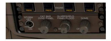
If it is daylight outside, then these will make little difference. The STORM switch provides a quick mechanism for turning all of the cockpit lights on to maximum brightness. It would be enabled if flying in poor weather to minimize the blinding effects of lightning flashes. Storm lighting is not modeled in the PMDG 747.
