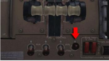
Repeat this process for engine 1. Pull the Start Selector, wait for N2 to reach the magenta line, set Fuel Control to RUN.
