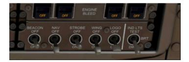
The external light controls are found in the lower right of the OVHD panel. We will not turn on the BEACON lights until we're ready to be pushed back or begin taxiing. The STROBE lights aren't turned on until we're ready to takeoff.
