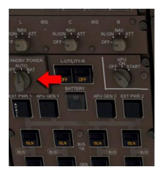
The switch is rotated to the right by right clicking on it. All switches are rotated to the left by left clicking.
