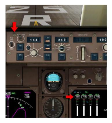
Apply slight forward pressure on the stick/yoke until you reach around 80 knots to keep the nose gear firmly against the runway. Use rudder to keep the plane centered on the runway. If something goes wrong or you receive an EICAS warning message, quickly return throttles to idle and initiate reverse thrust (F2 key). Autobraking will commence if you are travelling over 85 knots, otherwise apply braking, exit the runway, resolve the problem, and try again.
