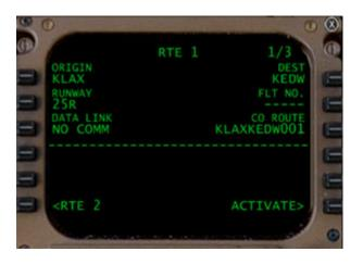
**Press LSK 6R (ACTIVATE) then press the EXEC button.** This will activate your flightplan and pass the relevant information to the flight control computer.
