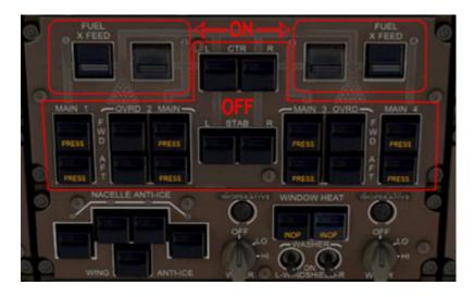
Disable NACELLE and WING ANTI-ICE Enable WINDOW HEAT
