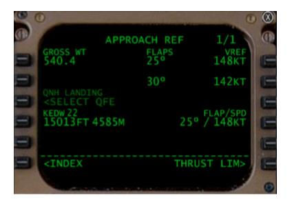
**Click the NAV/RAD button.** Note the heading as indicated next to LSK 4L. This is the heading for the landing runway. It should be 224 degrees for runway 22 at KEDW.
