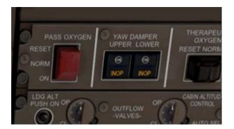
Yaw dampers automatically provide rudder and flight control input to aid the pilot and autopilot in maintaining smooth directional control. They help keep turns smooth and the passenger vomit off the apholstery. They should always be enabled during flight. The YAW DAMPER buttons are located at the top right of the OVHD panel. INOP is also displayed as the yaw dampers rely on hydraulic pressure to operate. Once the engines are started, they will remain ON and INOP will disappear.
