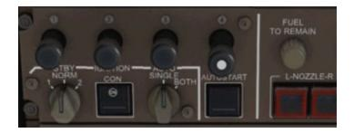
**Quickly open the throttle panel.** Watch the N2% RPM increase in the EICAS display. Bleed air from the APU is being 'blown' across the engine and is beginning to turn the turbines.
