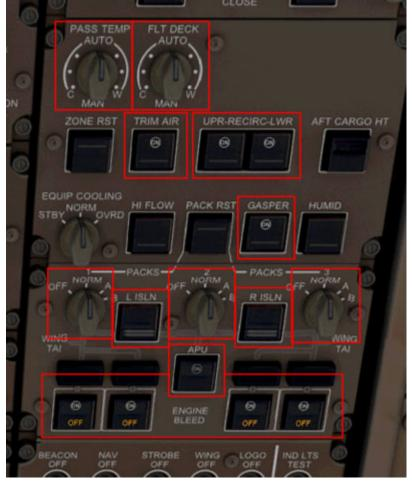
Air PACKS control the flow of air between the engines, the APU, the air conditioning system, and all other pneumatic systems. Setting them to NORM allows the pneumatic system to control the flow of air for all three air packs.
