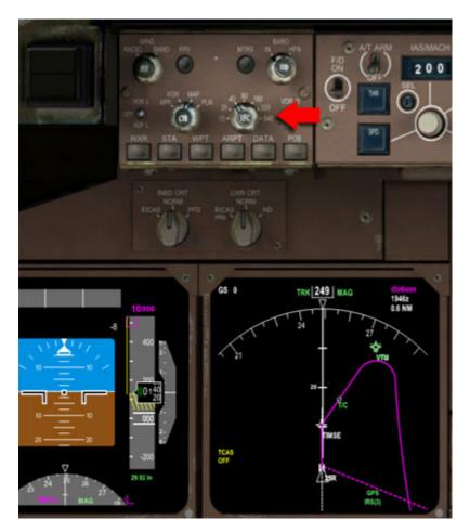
**Turn the F/D (Flight Director) ON.** When the autopilot is on, the Flight Director is what controls where your plane goes. When the autopilot is off, the F/D will give us visual cues as to climb pitch and bank angle to keep the aircraft flying safely.
